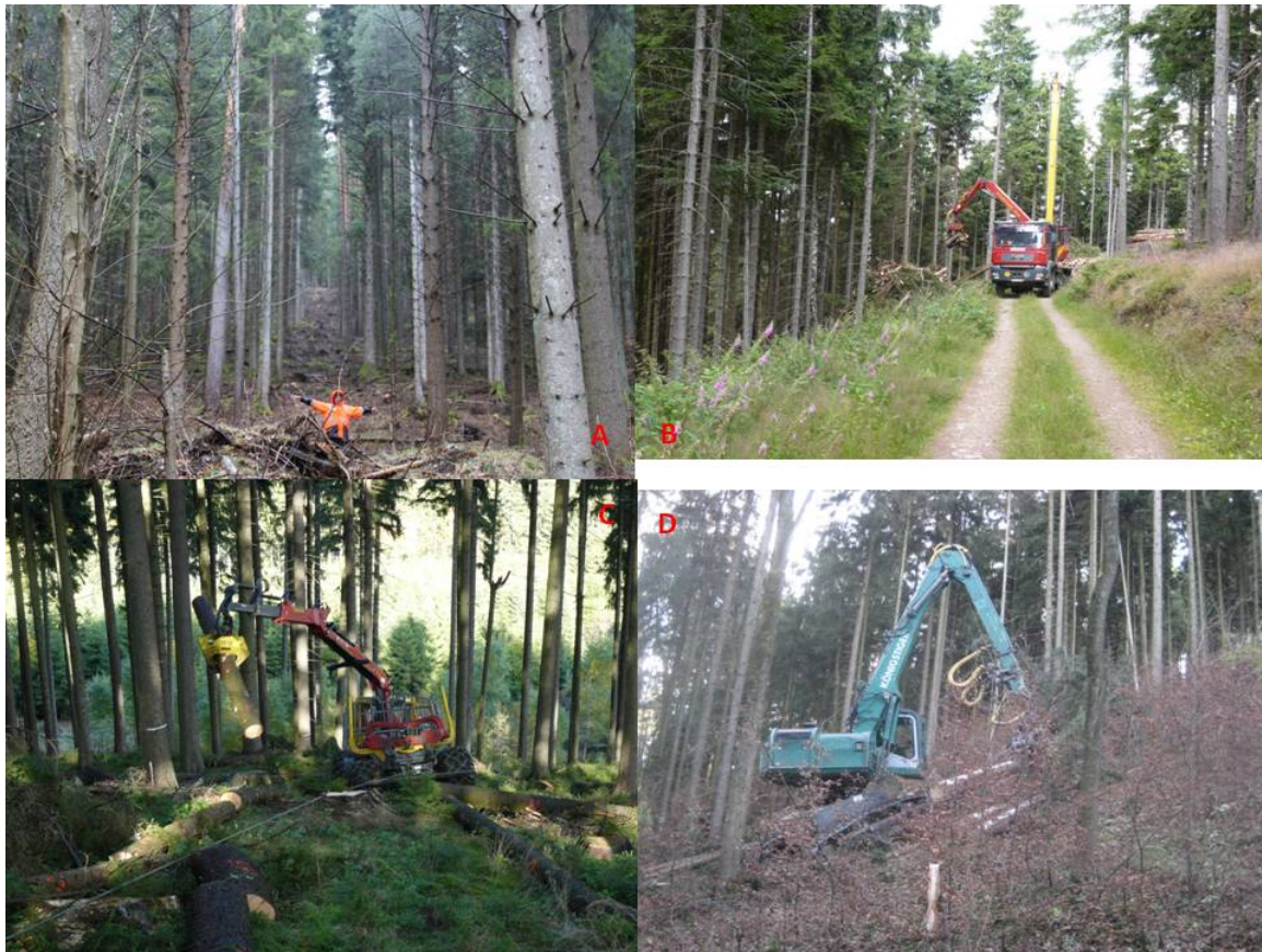
Figure 31 a, b, c, d: German harvesting: “gully-to-ridge” cable harvesting corridor (A); a truck mounted yarder with an integrated processor arm (B); a tethered wheeled (C) and tracked (D) harvester-processor. I note this looks like very easy terrain apart from perhaps A
