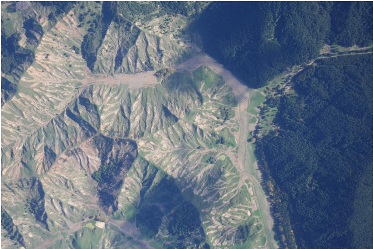
Figure 4: Contrast in shallow landslide damage on pasture and closed canopy exotic forest. Following storm April 2012, inland Wairoa. Photo courtesy of P. F. Olsens, Gisborne office.
