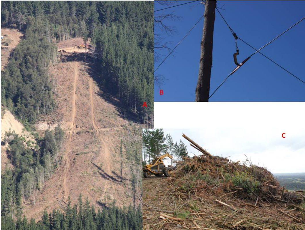
Figure 30 a, b, c: Chilean harvesting: “gully-to-ridge” setup around riparian zones (A); an intermediate support jack (B); a birdsnest of woody residue made up mainly of branches (C).
